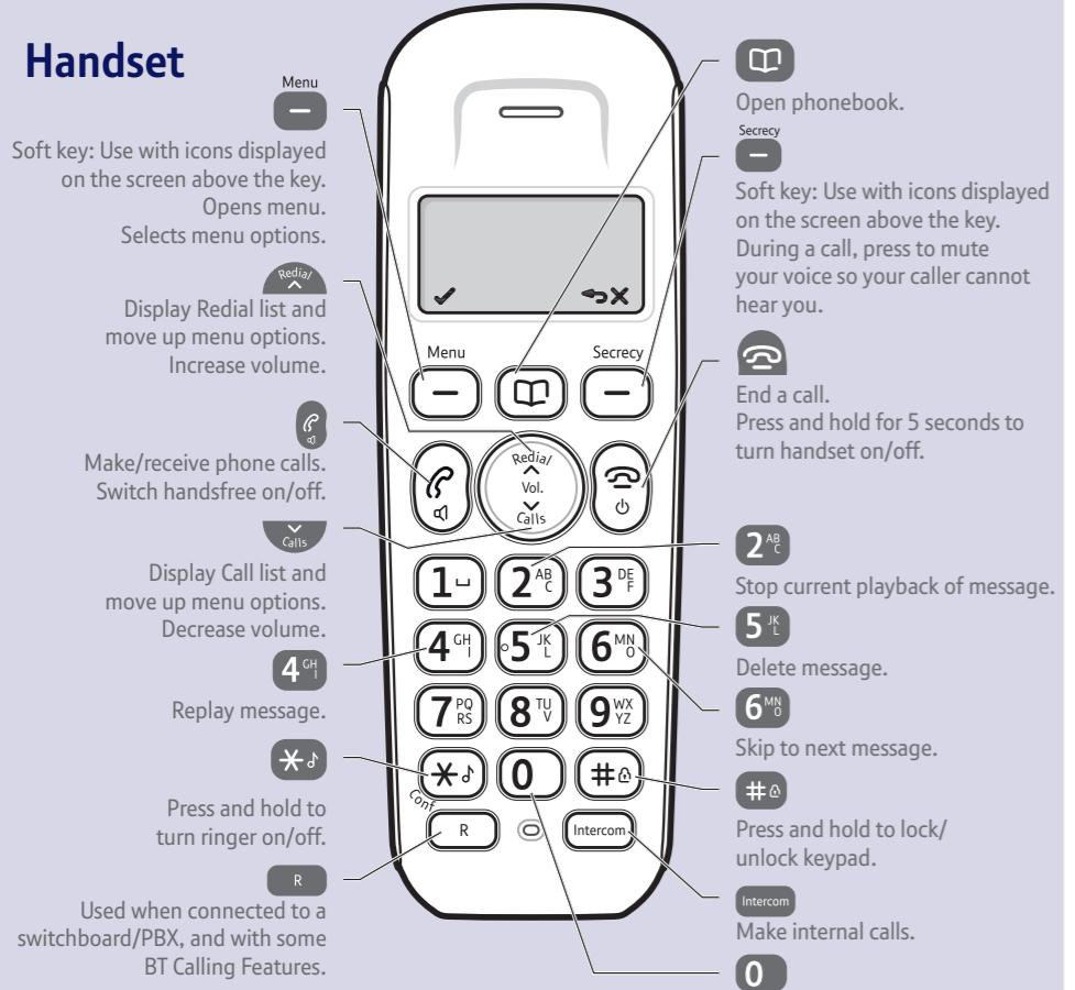
The answer machine handset controls on buttons **2<sup>AB</sup><sub>C</sub>**, **4<sup>GH</sup><sub>I</sub>**, **5<sup>JK</sup><sub>L</sub>** and **6<sup>MN</sup><sub>O</sub>** will only work when a message is being played on the handset.
